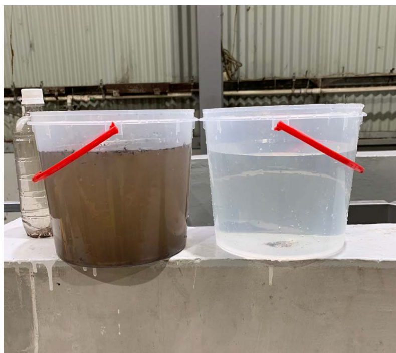
Figure 3 – shows an inflow and outflow sample from the Enviro EPS for visual comparison
