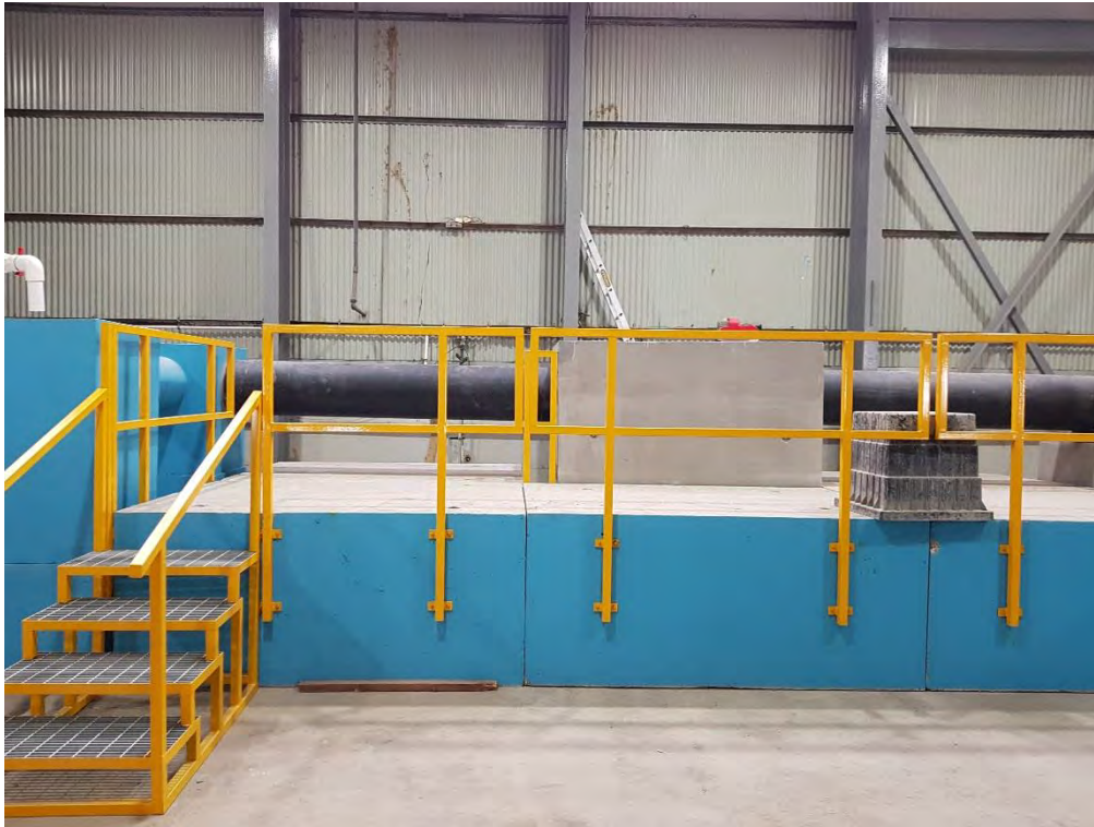
Figure 3 - Photograph of the oil/water separation test setup, showing the inlet pipework to the treatment chamber (at centre)
