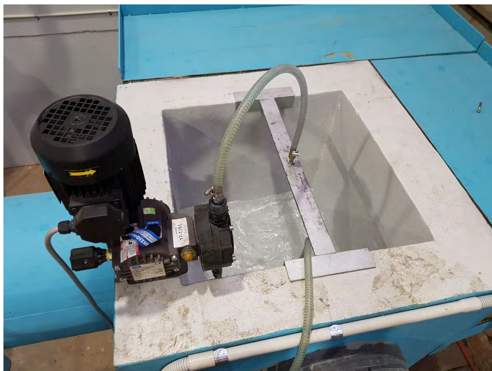
Figure 5 – Detailed view of the oil/water mixing pit upstream of the treatment device
