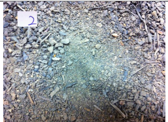
Figure 16: Soil sample 2. Note large presence of fines or "dust".
