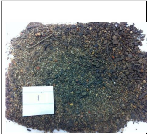
Figure 5: <math><2.36\text{ mm}</math> homogenous sample
