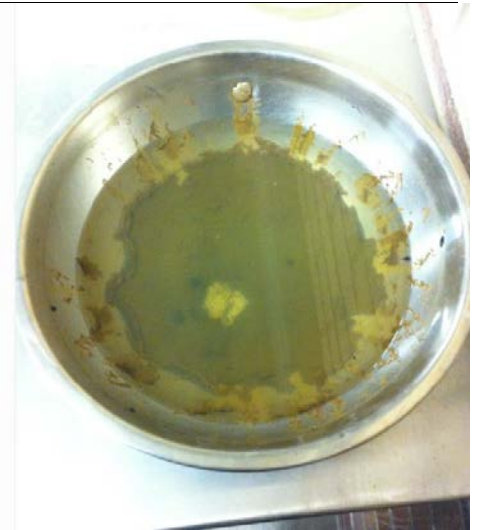
Figure 7: Fines settled from suspension (pre-siphoning)
