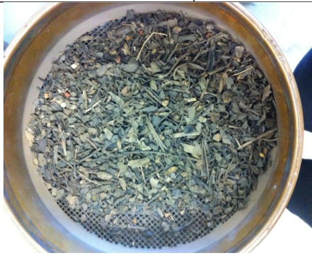
Figure 15: >2.36mm fraction removed from 24 hour time dependant experiments. Note the presence of plant material (dried leaves, twigs, seed pods)
