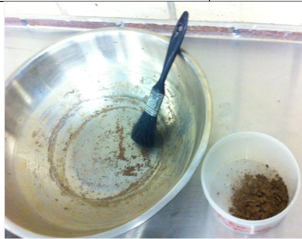
Figure 9: Supernatant water siphoned and evaporated leaving fines.
