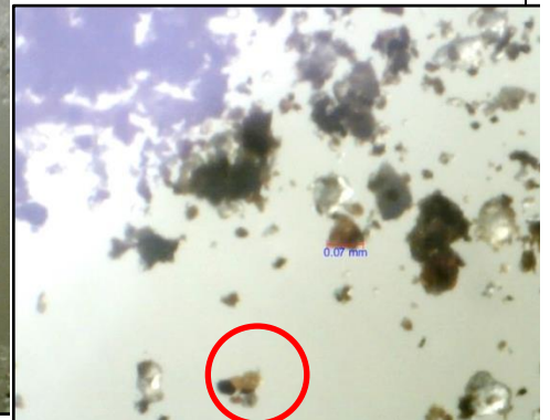
Figure 12: Feldspar minerals in <math><75\mu\text{m}</math> fraction at 390 x magnification
