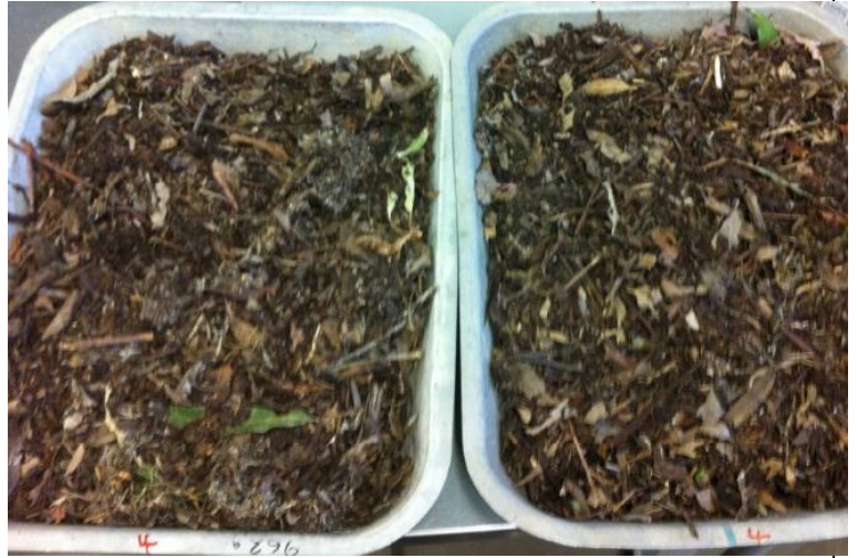
Figure 30: Oven drying of sample four. Note fresh green vegetation in sample not yet undergone decomposition
