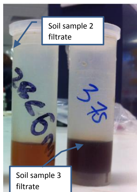
Figure 19: Filtrate from Soil sample 2 and 3. Note Soil sample 2 had a lot of humic acid (indicated by brown color), and Soil sample 3 had even more so.
