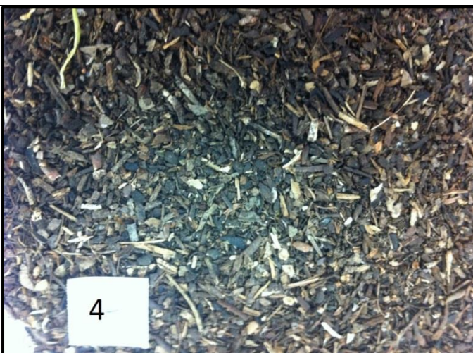
Figure 33: >2.36 heterogeneous fraction used for 24 hour experiments
