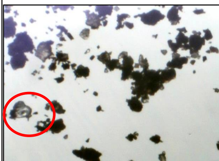
Figure 10: Quartz minerals in <math><75\mu\text{m}</math> fraction at 390 x magnification
