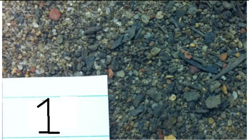
Figure 14: Macroscopic minerals present in >2.36 sample at 0 magnification
