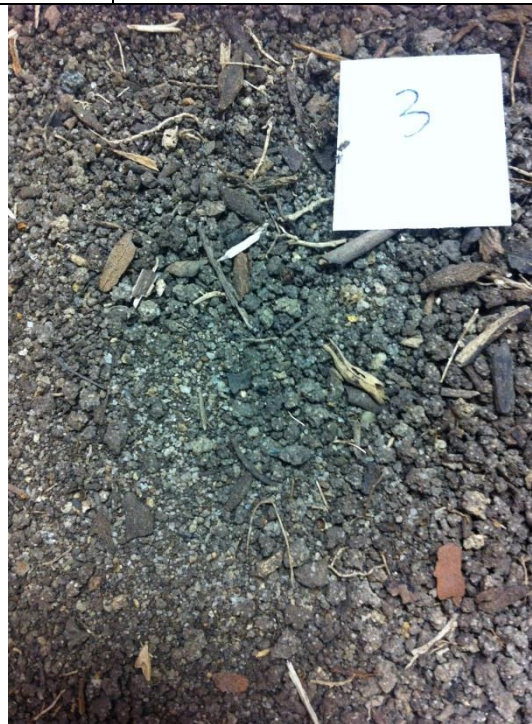
Figure 20: Soil sample 3 as in-situ. Red highlights presence of living vegetation in sample.
