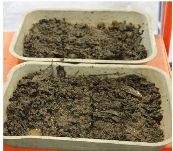
Figure 4: Drying of soil sample in 180°C oven
