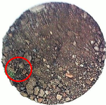
Figure 20: Soil sample 3 as in-situ. Red highlights presence of living vegetation in sample.
