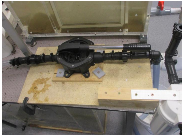
Figure 25: Hand held pump used to create a wet vacuum to suck particles out of each compartment
