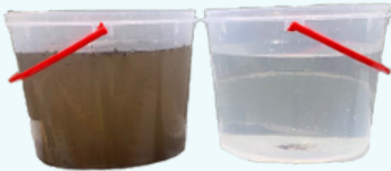
(Left) Natural Stormwater (Right) Results after single pass in Enviro H45
